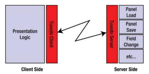
Figure 2-3. Tuxedo connects the client to the functions in the server process.
