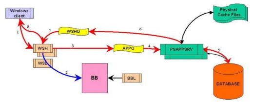
Figure 2-8. A simplified three-tier Windows client transaction
