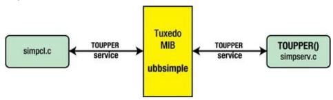
Figure 2-4. The Simple client and application server
