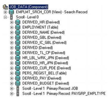
Figure 5-3. JOB\_DATA component structure from Application Designer<sup>7</sup>
