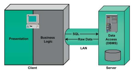
Figure 1-3. The original client/server model
