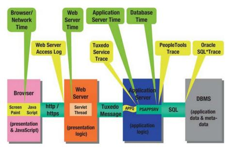
Figure 10-6. Ping measurements on the PIA infrastructure
