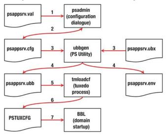
Figure 12-1. Configuration processes and files
